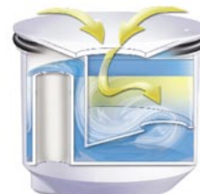
urine passes through the sealant...
